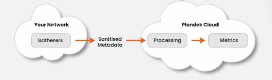
Plandek offers clients the option of an **on-premise data gatherer**. This option ensures that sensitive data (received automatically via the connected APIs and not required by Plandek) are removed from the dataset before its encrypted export into the cloud - and therefore such data never leaves the client's network.
